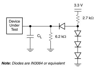
Figure 11. Test Setup
