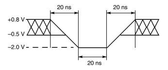
Figure 7. Maximum Negative Overshoot Waveform
