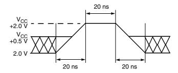
Figure 8. Maximum Positive Overshoot Waveform
