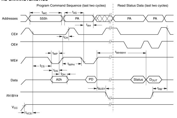
**Note:**  $PA = program \ address, \ PD = program \ data, \ D_{OUT}$  is the true data at the program address.
