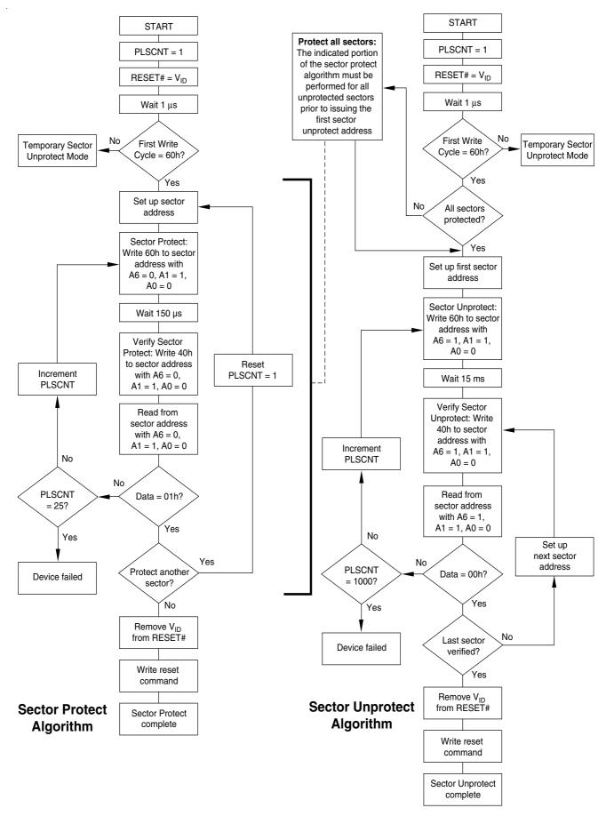
Figure 2. In-System Sector Protect/Unprotect Algorithms
