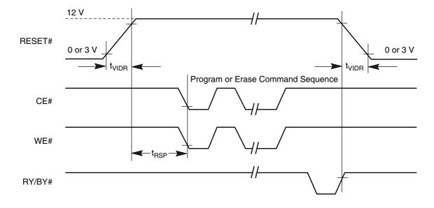
Figure 20. Temporary Sector Unprotect Timing Diagram
