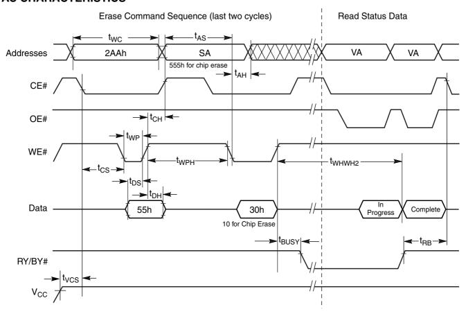
**Note:** SA = sector address (for Sector Erase), VA = Valid Address for reading status data (see "Write Operation Status").
